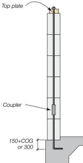
Table 15.2 provides ultimate racking capacities of reinforced 150mm and 250mm Hebel® PowerBlock™ walls. The reinforcement is N12 bar or 12mm threaded rod at nominal 1000mm centres. The reinforcement must be tied to the footings and wall top plate through the bond beam.
