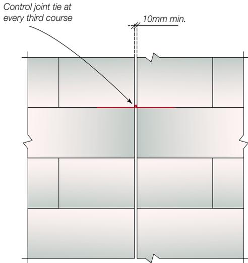
**Fig 14.22 Hebel® PowerBlock™ work Typical Movement Joint Detail (plan)**
