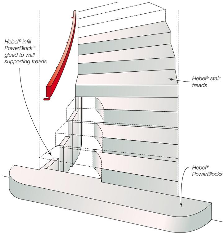
Fig 14.37 Stair Tread Set-Out (isometric)
