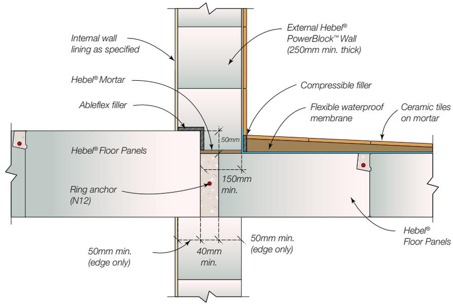
**Fig 14.34 Deck Connection Detail (side elevation)**
