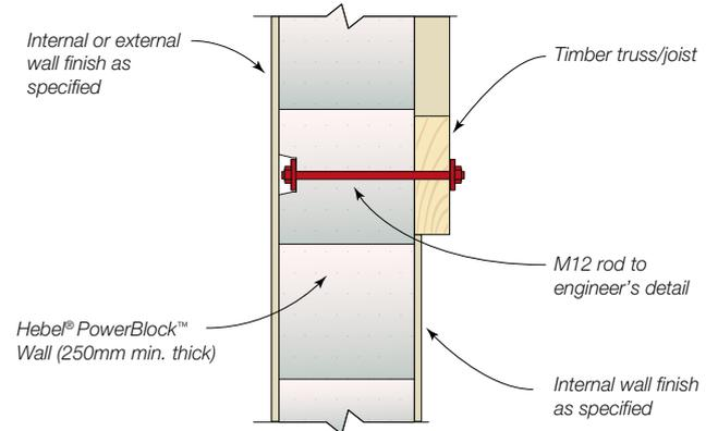
**Fig 14.11 Truss Spanning Over Non-Load Bearing Hebel® Walls (elevation)**
