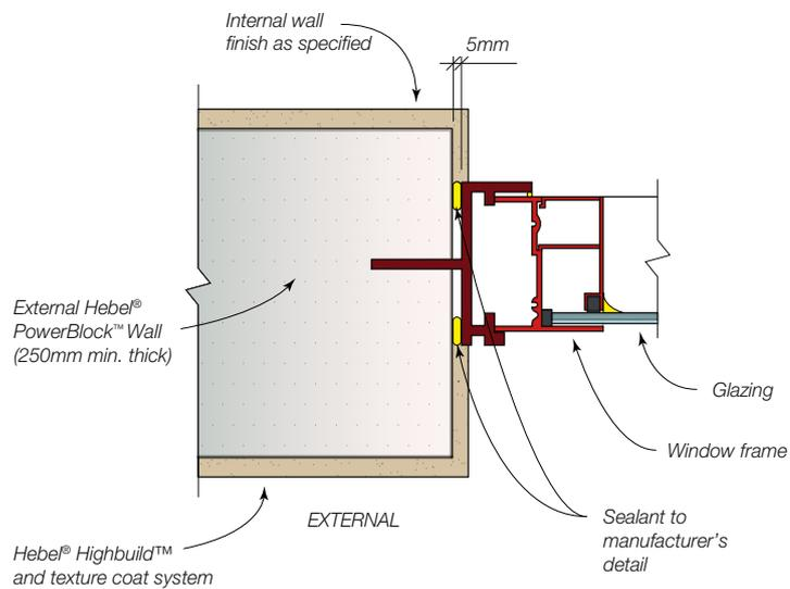
**Fig 14.45 Aluminium Window Frame - Window Head Detail (elevation)**
