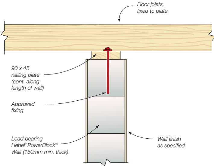
**Fig 14.12 Timber Truss/Joist Fixed to Hebel® Walls (elevation)**
