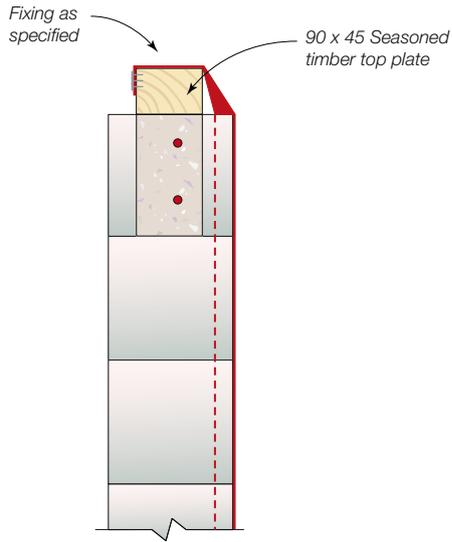
**Fig 14.6 Roof Top to Plate Fixing to Hebel® Wall - Strap (elevation) - for typical trussed roof**
