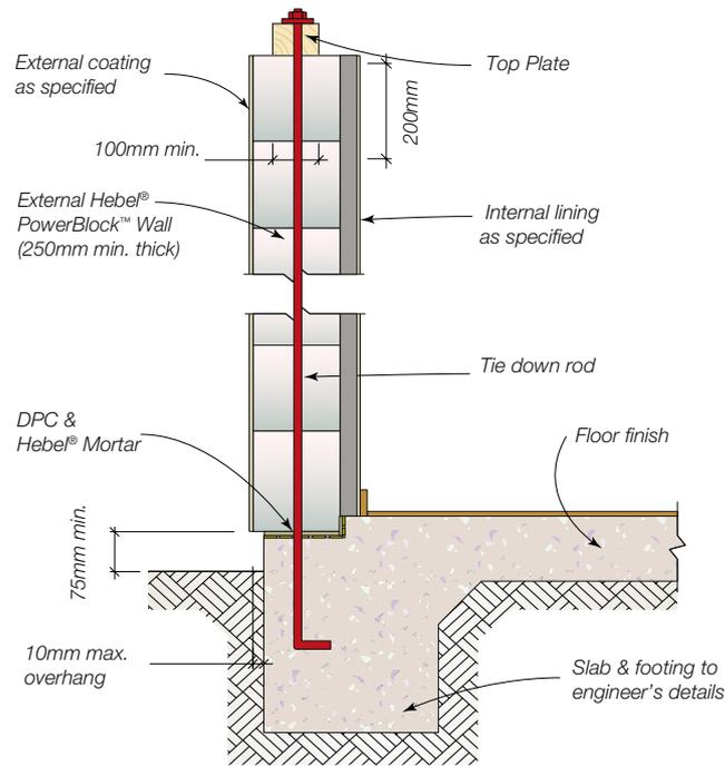
Fig 15.7 Concrete PowerBlock™ Sub-Floor Detail (elevation)
