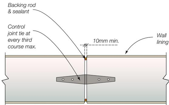
**Fig 15.18 Hebel® PowerBlock™ work Typical Movement Joint Detail (elevation)**
