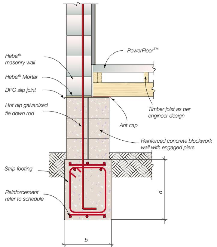
Tie down rods/engineering restraints must be embedded into the footing and pass up through the sub floor and into the Hebel PowerBlock™ work.
