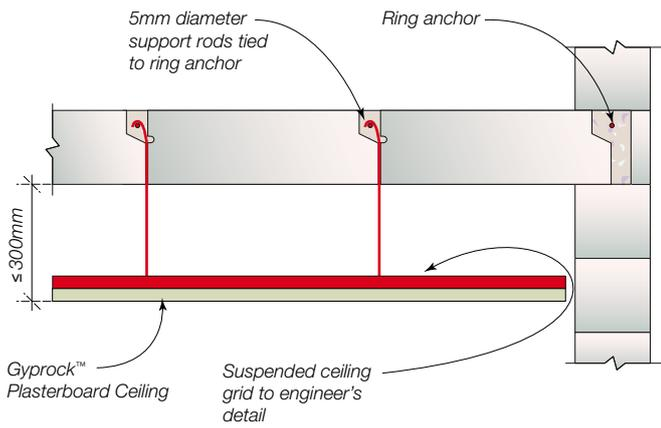
Fig 14.31 Ceiling Support Detail B (isometric)
