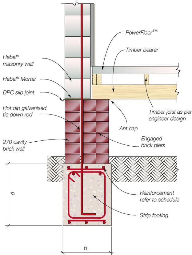
Fig 15.2: Strip Footing, Concrete PowerBlock™ Sub-Floor
