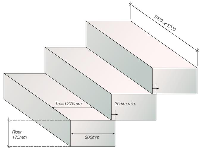
Fig 14.38 200mm wide x 50mm thick Hebel® PowerBlocks adhered to walls on their ends to provide support for treads (isometric)
