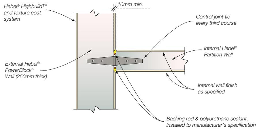
Fig 14.16 External Corner with Control Joint (plan)
