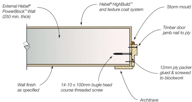
**Fig 14.42 Timber Door Frame (Internal) to Hebel® Wall Fixing (plan)**
