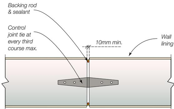
**Fig 14.21 Hebel® PowerBlock™ work Typical Movement Joint Detail (elevation)**
