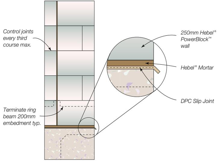
Fig 14.19 Typical Control Joint - plan
