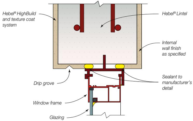
**Fig 14.46 Lintel Installation**
