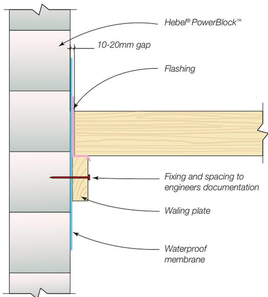
**Fig 14.35 Deck Connection Detail (front elevation)**
