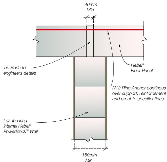
Fig 14.30 Ceiling Support Detail A (elevation)
