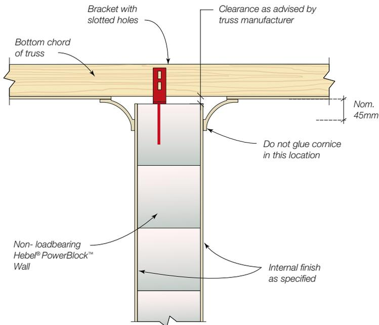
**Fig 14.13 Tiled Roof Eave and Hebel® Wall Junction (elevation)**
