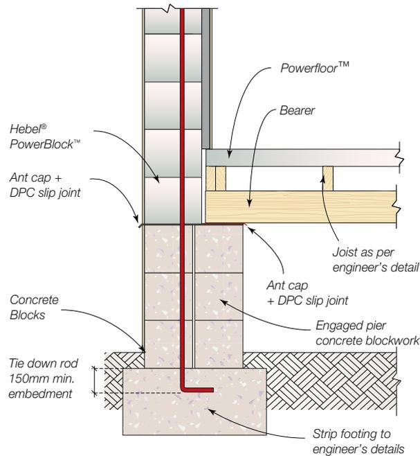
**Fig 15.8 Double Brick Sub-Floor Detail (elevation)**
