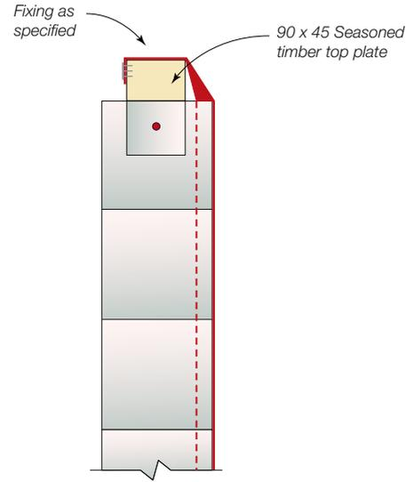
**Fig 14.7 Strap Fixing to Hebel® Walls (isometric - typical trussed roof)**
