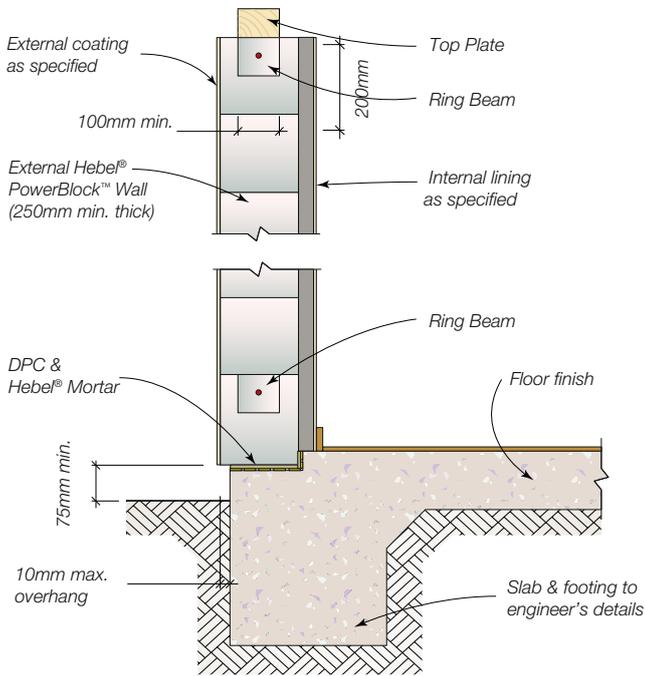
**Fig 14.3 Internal Load Bearing Hebel® PowerBlock™ work on stiffened raft slab foundation (elevation)**
