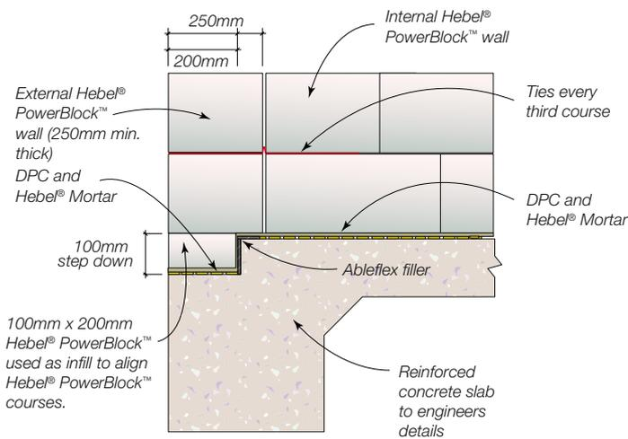
**Fig 14.4 Concrete PowerBlock™ Sub-Floor Detail (elevation)**
