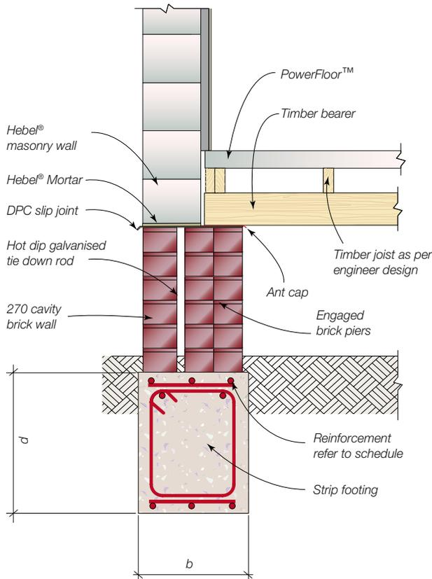
**Fig 7.1.4: Strip Footing, Concrete PowerBlock™ Sub-Floor**
