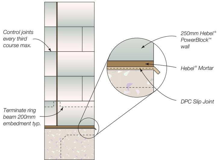
**Fig 15.17 Typical Control Joint - plan**
