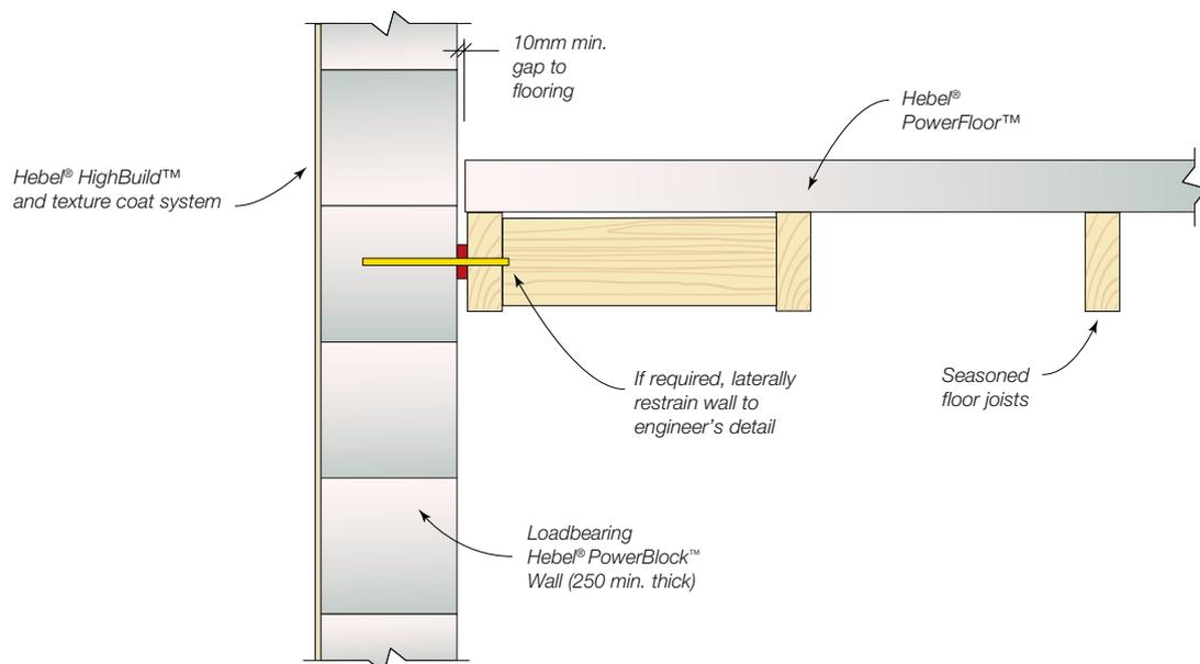
**Fig 14.28 Timber Floor Support Detail (elevation)**
