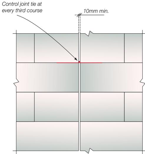
**Fig 15.19 Hebel® PowerBlock™ work Typical Movement Joint Detail (plan)**
