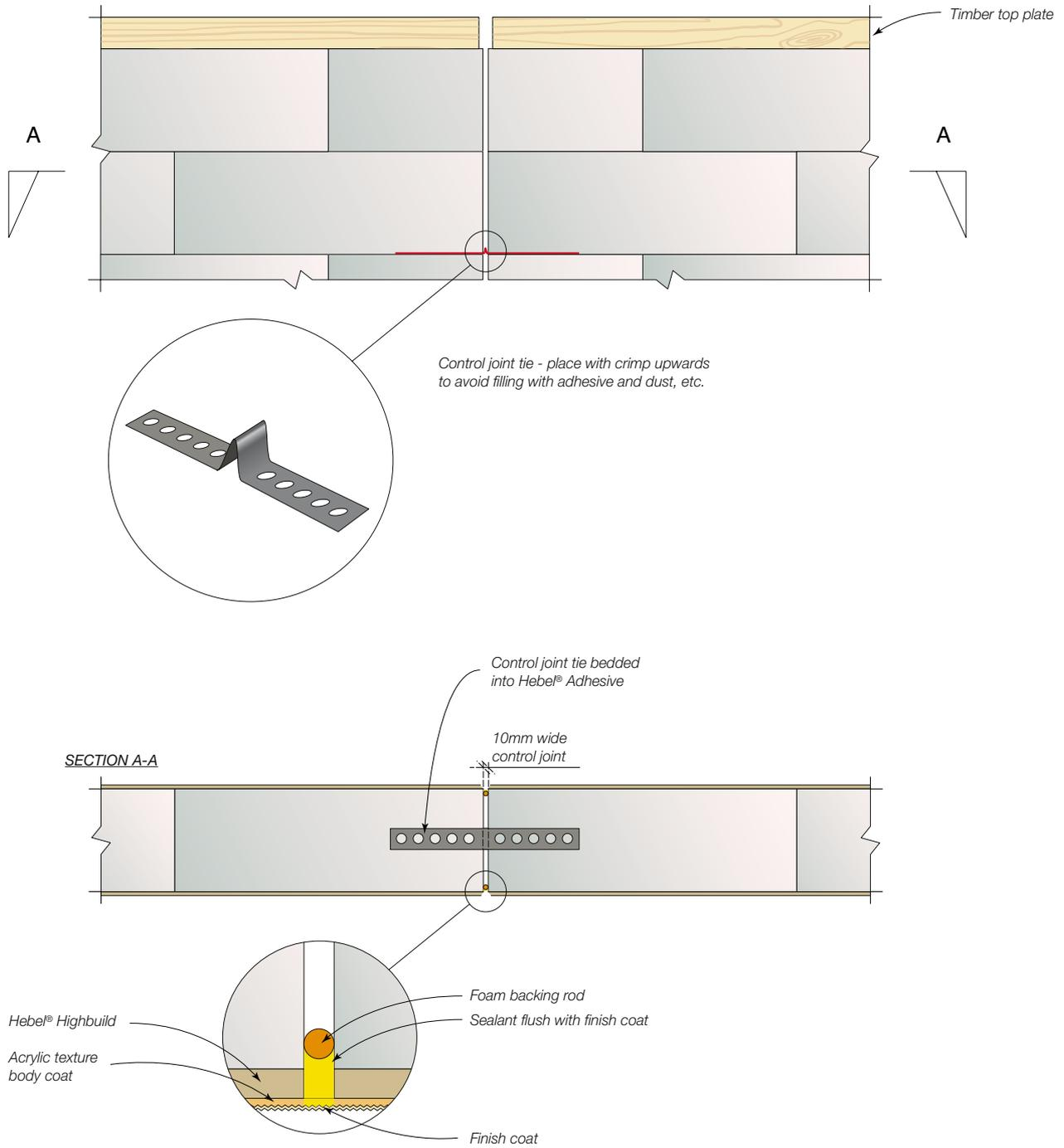
**Fig 15.15 Typical Bond Beam Control Joint - elevation**
