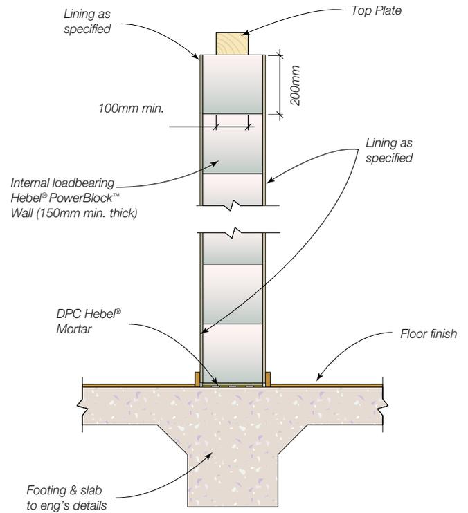
**Fig 14.2 Hebel® PowerBlock™ work showing infill block to slab rebate (elevation)**
