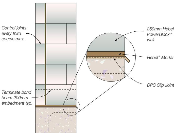
**Fig 15.16 Typical Ring Beam Control Joint - elevation**
