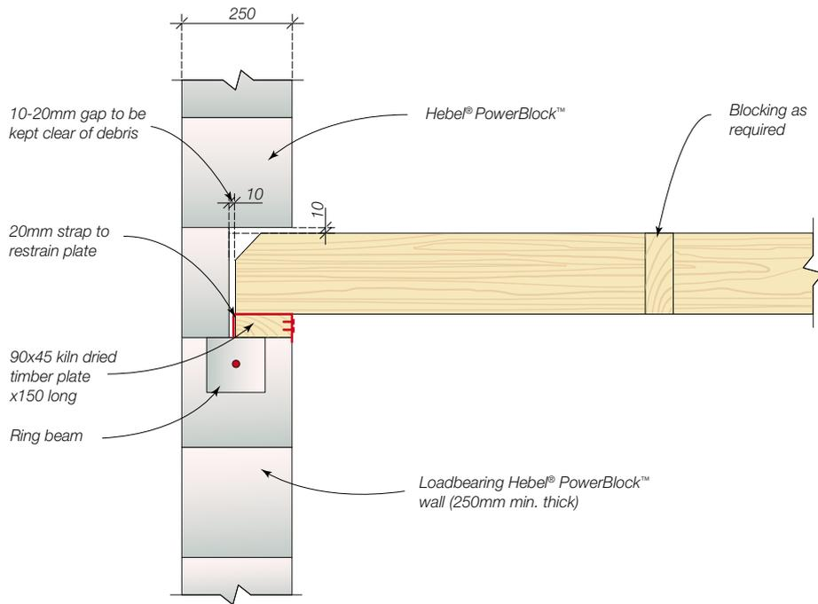
**Elevation - Floor Joists to External Wall**
