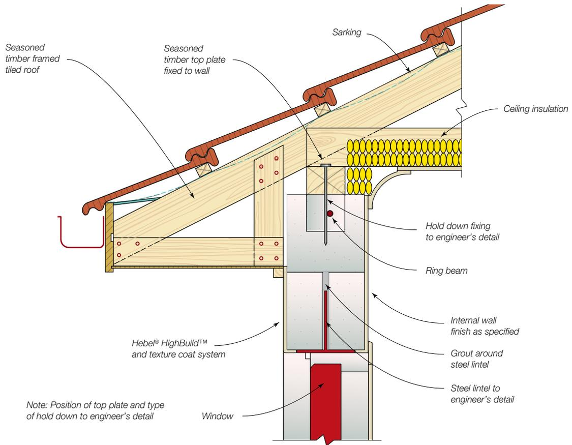
**Fig 14.14 Vaulted Ceiling & Roof Top Plate Fixing To Hebel® Wall (elevation)**
