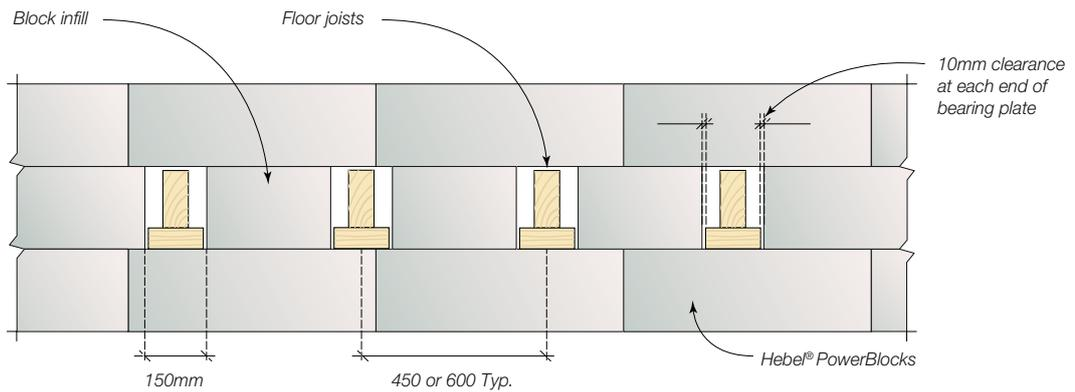
**Fig 14.29 Hebel® Flooring Panels using Ring Anchor Construction on Load Bearing Interior Wall (elevation)**
