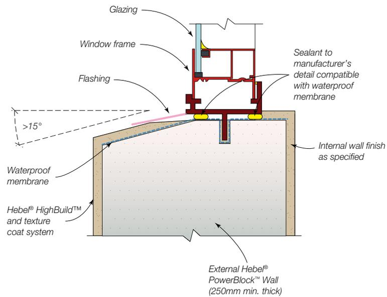
**Fig 14.44 Aluminium Window Frame - Window Jamb Detail (elevation)**
