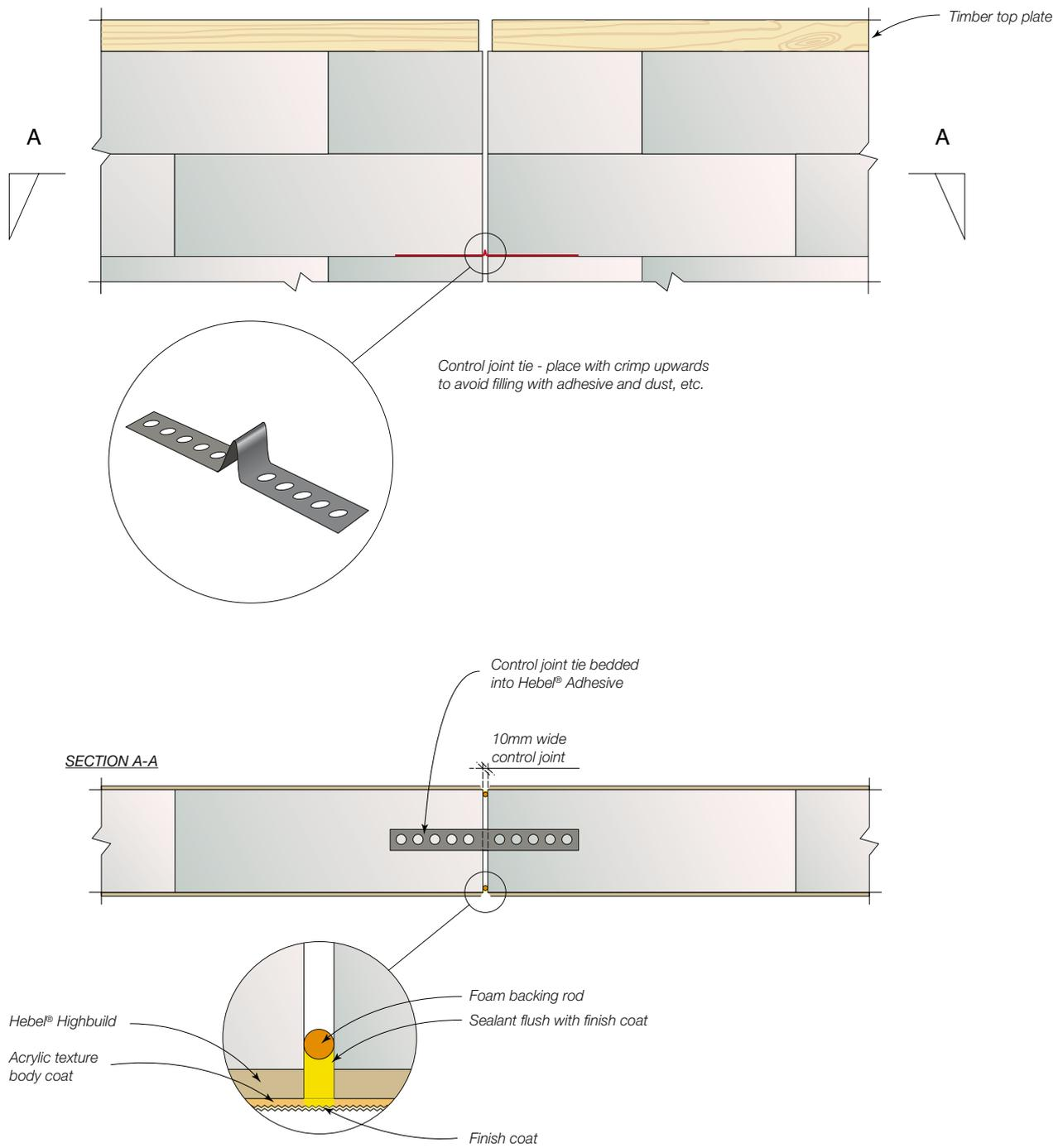
Fig 14.18 Typical Bond Beam Control Joint - elevation
