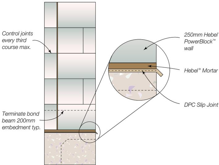
Fig 14.20 Typical Ring Beam Control Joint - elevation
