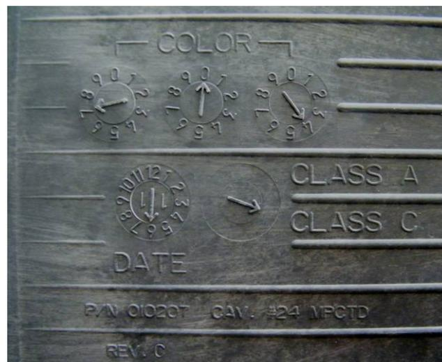
Plate 2: Rear view of tile showing manufacturing date and colour batch details.
